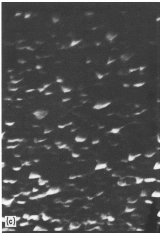
*Figure 4* Scanning electron micrographs of cadmium film grown on different substrate: (a) glass (b) few atomic layers of titanium on glass. Original magnification: (13 440 X). (c) Mica, original magnification: (16 800 X).
